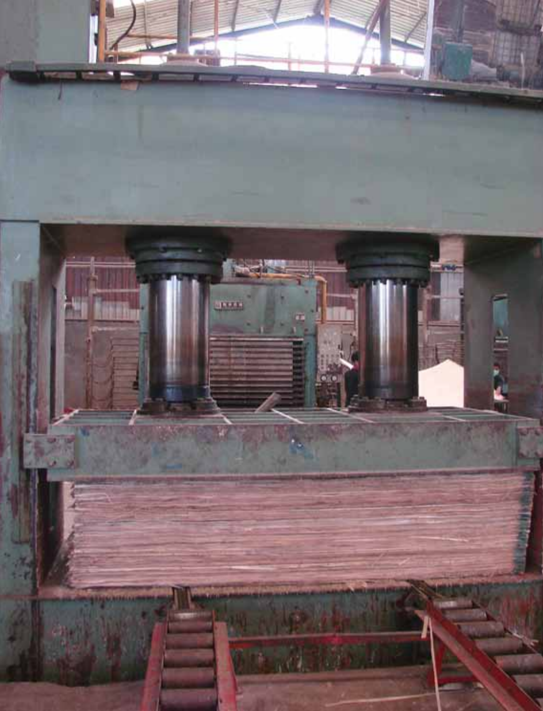
Mill in Cianjur state, Java Island, pressing during the process of producing plywood
