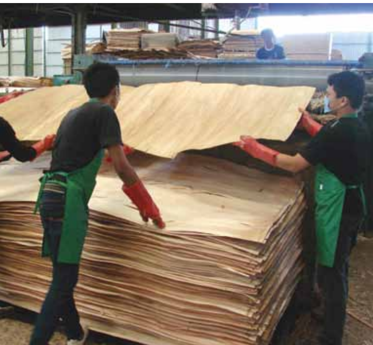
Gluing of veneer sheets at a mill in Cianjur, Java
