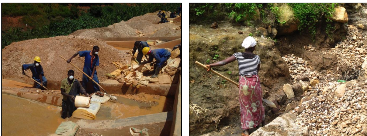
Photos 6 and 7: Ground sluicing of 3T ore is common throughout the GLR
